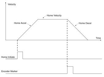
*Figure 33: Home to Marker Profile (Calculated Offset)*
